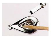
19 Remove tongue. Spread thin, even layer of glue in recessed area avoiding hole at bottom. Do not flood with glue as it will seep into hole and cause a blockage.
